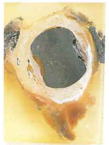
Fig. 10: Cross section through the shank of a hip endoprosthesis cemented in the femur.
